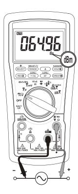
**Note:** In **dBm** function, power up default reference impedance will be displayed for 1 second before displaying the dBm readings. Press **dBm-\Omega** (**RANGE**) button momentary to select different reference impedance of 4, 8, 16, 32, 50, 75, 93, 110, 125, 135, 150, 200, 250, 300, 500, 600, 800, 900, 1000, up to 1200 $\Omega$ . Last selection
