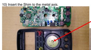
Very Important !! Round Recess on the Shim must be facing upward.
