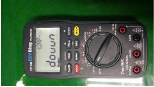
16-3) When the Downloading is completed, the Meter will display Software Version number.
