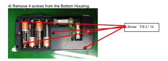
5) Open the Bottom Housing and Remove the Fuse (11A).
