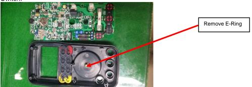
8) Remove the Rotary Switch from the Top Housing.
