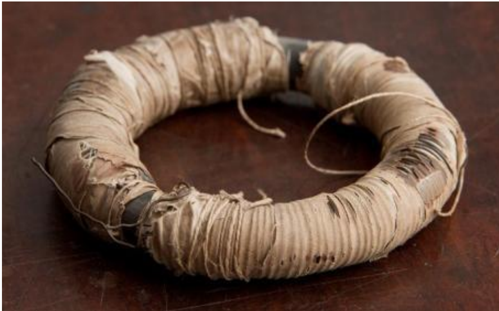
Faraday's toroidal transformer – the first on record (Picture courtesy of IET)
