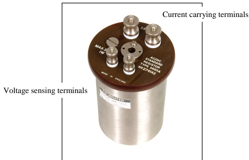
Fig. 1.1 The "Wilkins" type transfer standard 2TP resistor (designed for immersion in a temperature controlled bath of mineral oil - courtesy ASL U.S.)
