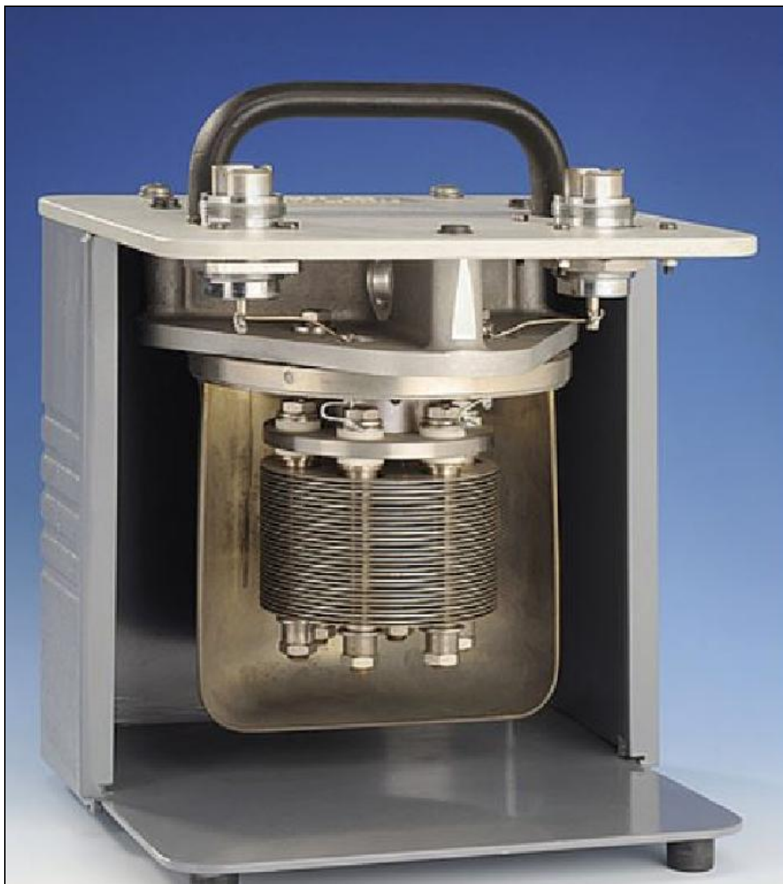
Fig. 5.3 The internal construction of a 1nF transfer standard
