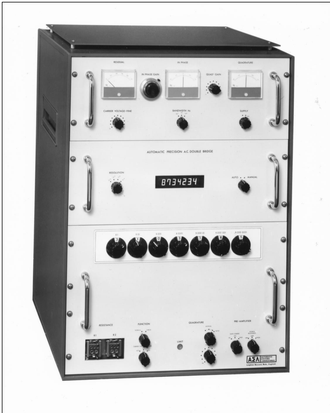
Fig. 2.1.2 The A7 employing two seven decade dividers (Picture courtesy ASL Ltd). (N.B. weight about 70kg!)
