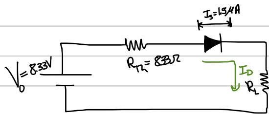
$$I_D = I_s e^{\frac{V_o}{0.026}} = 1.5\text{ }\mu\text{A} e^{\frac{8.33\text{ V}}{0.026}} =$$
