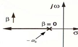
A single pole cannot contribute a phase shift greater than  $90^\circ$  and the system is unconditionally stable for all non-negative values of  $\beta$ .
