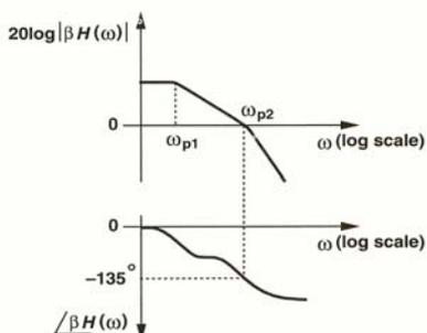
Since  $\angle \beta H$  reaches  $-135^\circ$  at  $\omega = \omega_{p2}$ , the phase margin is equal to  $45^\circ$ .
