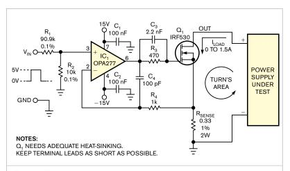
Figure 1 This simple current sink allows you to test both the static and the dynamic behavior of power supplies.
