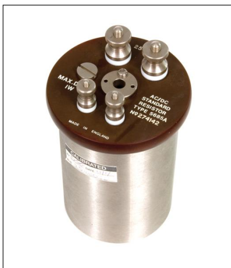
Fig. 1.5.1 A Wilkins type reference resistor
