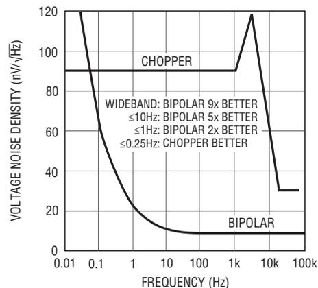
**Figure 1. Bipolar vs Chopper Noise Comparison**
