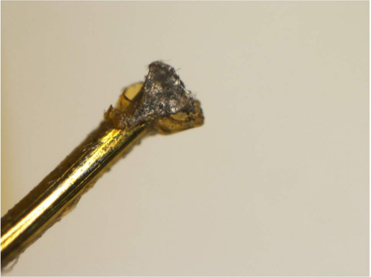
Evanohm resistor wire end
