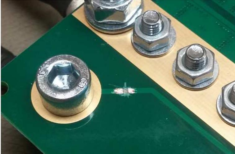
2. Solder a 10 ohm resistor (0805 package) onto the created pads.
