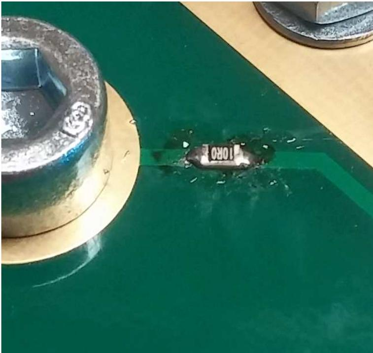
3. Measure the resistance with a multimeter to avoid a possible short circuit.
