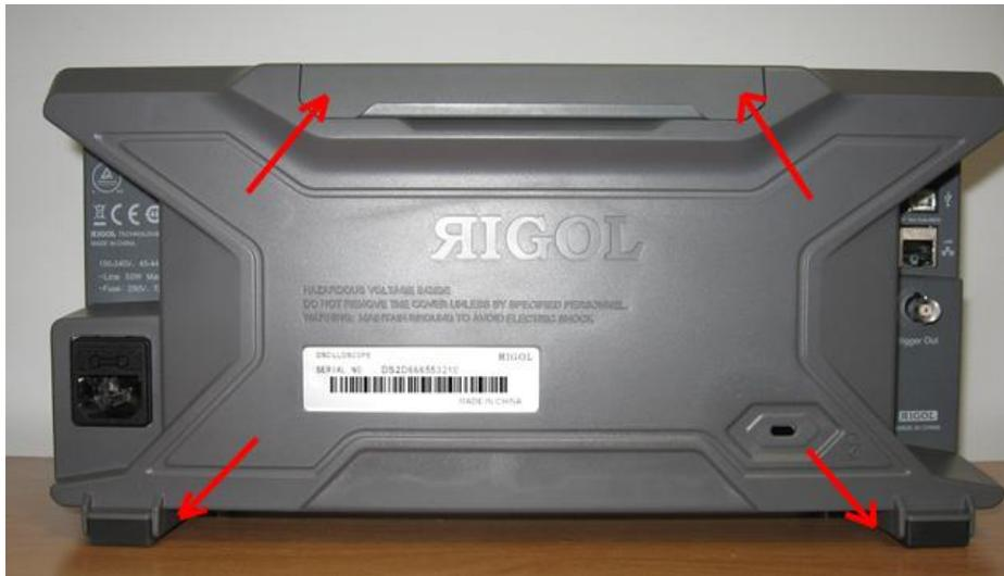
Also the metal screen with the power supply has to be removed. It is held by (if I remember correctly) 8 Torx screws at the top and bottom. Also requires removing the nut holding the BNC Trigger Out connector. Once the back cover is separated a bit, the power supply connectors can be unplugged from the motherboard and the power supply can be put aside. I placed a towel on the desk to protect the scope front panel and controls from been scratched accidentally.
