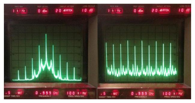
So orientation of the inductors did matter. I figured out from the slope of the VCO control voltage that the VCO was running lower in frequency with the inductors soldered in parallel orientation. Therefore the overall inductance was higher than with inductors at right angle. On the other hand, the left picture with the parallel inductors looked better, and since it was with a higher inductance then perhaps I needed to try even larger inductance. I did not have a 3nH inductors so I tried 3.3nH:
