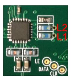
What can be possibly wrong with them? Well, an RF person would tell right away that they should have been positioned at right angle to reduce coupling. Same says the PLL Datasheet: ... "To reduce mutual coupling, the inductors should be placed at right angles to one another." I always place any adjacent inductors at right angle. Any RF designer would. Not Yaigol Yingineers. All they needed to do is to read the Datasheet. They did not. Neither they had a clue about the basics of RF design.
