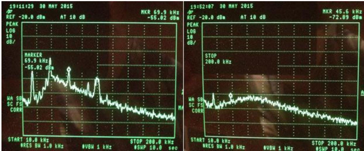
That resulted in the hump disappearing at LDO output. Here is the final PLL LDO output rail spectral screenshot, nice and quiet:
