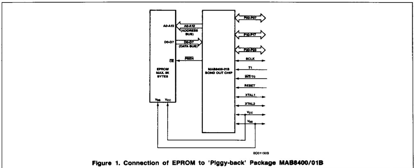
Figure 1. Connection of EPROM to 'Piggy-back' Package MAB8400/01B
