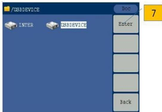
7. Select the downloaded firmware file by rotating the general purpose knob, and then push the Execute bezel button.
