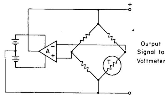
Fig. 1. Self-balancing Wheatstone bridge.
