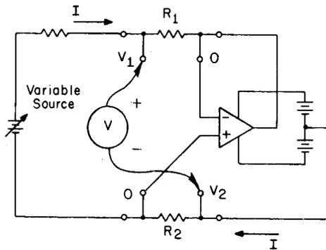
Fig. 2. A method for intercomparing two four-terminal resistors.
