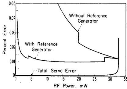
Fig. 5. Voltmeter errors with and without offsetting reference voltage generator. Total servo errors with bias currents of 6 nA and amplifier offsets of 10  $\mu$ V.
