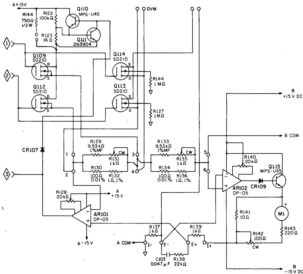
Fig. 8. Self-balancing current loop. The bolometer is connected to the terminals identified by  $I-$ ,  $E-$ ,  $E+$ , and  $I+$ .
