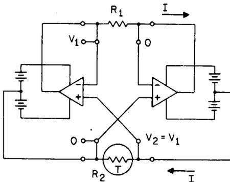
Fig. 3. A self-adjusting current loop.
