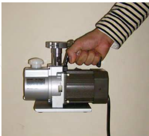
Fig. 5. A small rotary vacuum pump.
