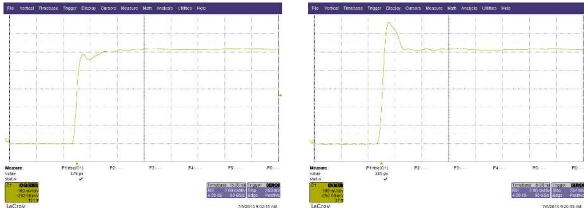
So, with light capacitive load (active probe) it apparently does a hefty 345ps. It can almost compete with the picosecond pulser (~200ps), and this is just a microcontroller's GPIO pin. Thanks for that, NXP :-)
