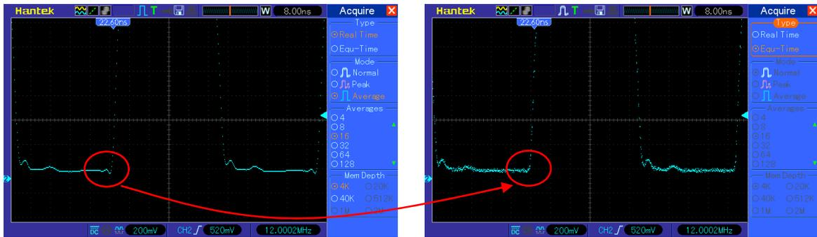
Knowing this and choosing “equ-time” mode from now on, I can be sure that when I see a signal with ringing, it would be either my signal source, or the analog part of the scope.
