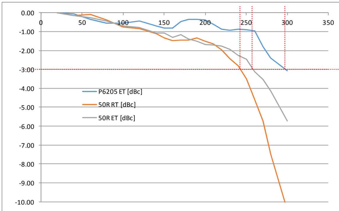
The bandwidth limitation effect caused by the post-filter can easily be seen. I would be interested if someone could make more precise measurements, to see if that -1dB between DC and 200MHz is real, or is a measurement error of mine / the miniVNA.
