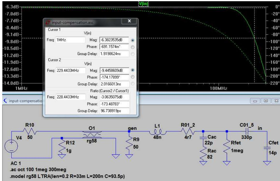
When driven from 50 ohms, this particular step fully compensated for the large input inductance, but it also increased capacitance at high frequencies. This in turn impaired passive probe matching.
