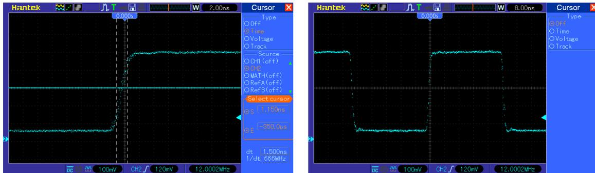
Tektronix P6205 active probe (750MHz / 2pF) (used @ ebay ~ 50USD), 50 ohm termination at scope input (BNC-t + 50 ohm stub):
