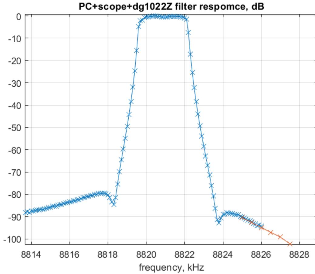
Here blue crosses show data points obtained by averaging 10 scope waveforms, and the red crosses require averaging of 100 scope waveforms by PC
