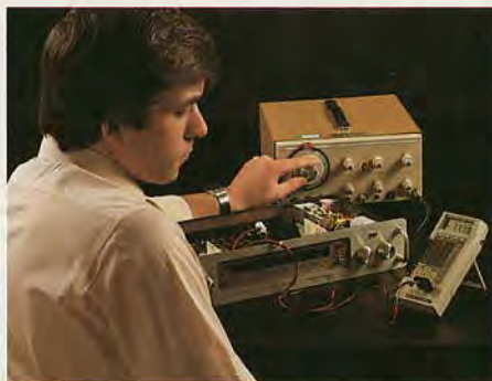
Combined frequency and dB capabilities of the 8060A make it ideal for audio applications...from testing multistage amplifier gain to checking filters, tone controls, equalizers and attenuator pads.
