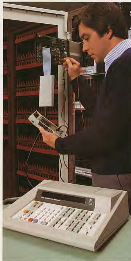
Analog and digital servicing go hand-in-hand with the 8060A DMM and the 9010A Micro-System Troubleshooter. The Fluke 9010A uses automatic tests to check a micro-system's RAM, ROM and I/O. It's the first tester designed specifically for troubleshooting digital systems.
