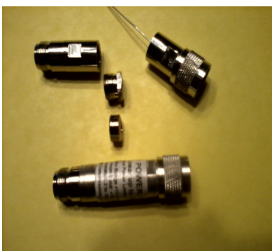
'N' connectors before (top), and after final assembly (bottom) with a label applied. This construction technique also applies to other 'clamp' solder connector types.
