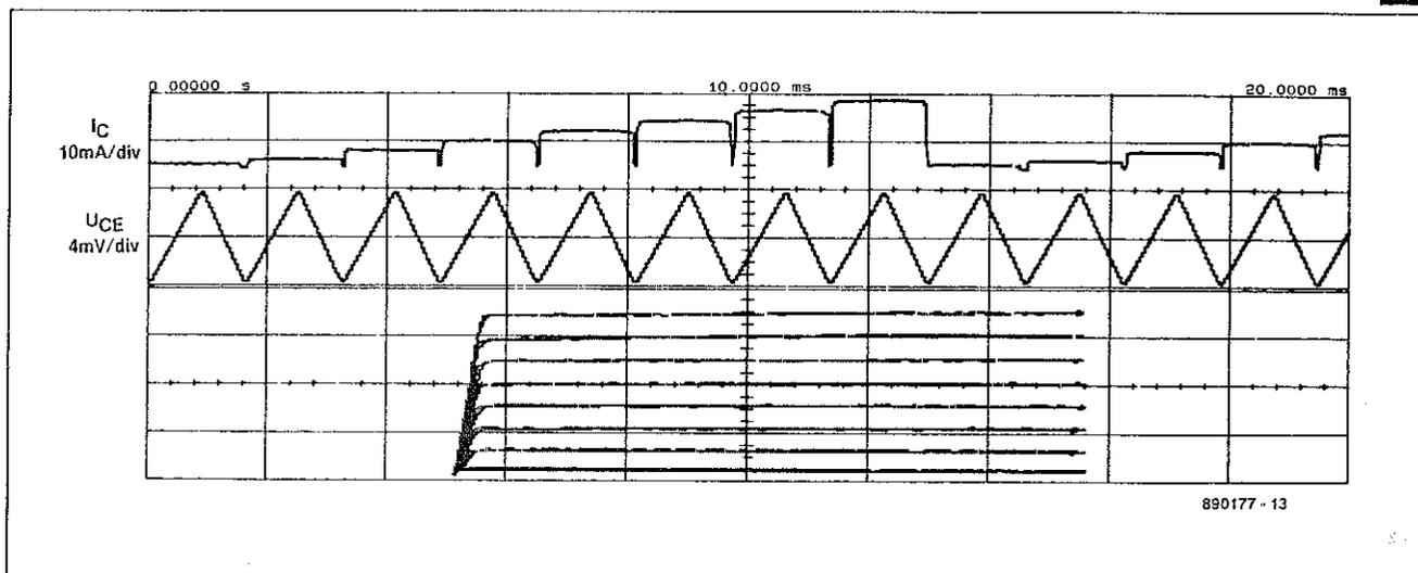
Fig. 4. Screenshot provided by a Hewlett-Packard digital oscilloscope to illustrate the operation of the transistor curve tracer.
