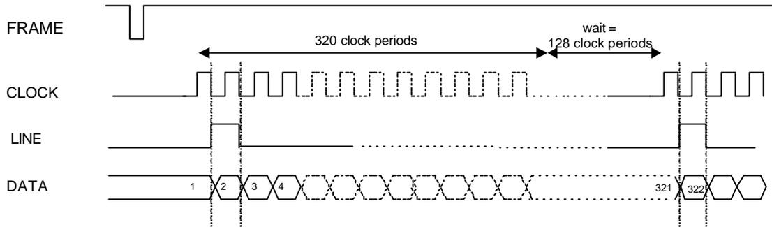
Frame signal is asserted low at the beginning of each frame.
