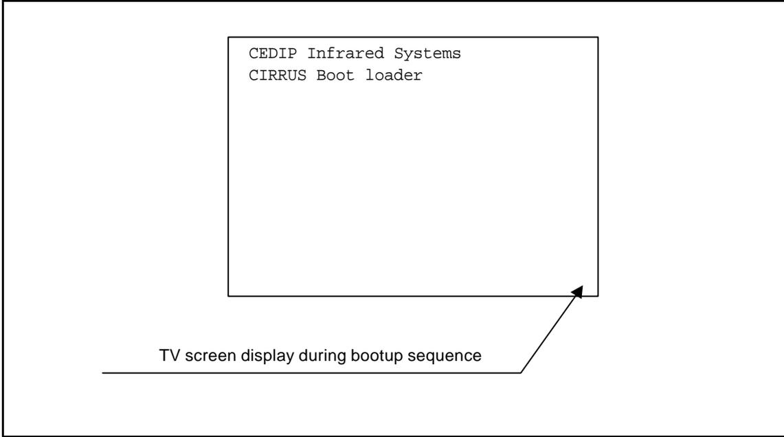
During this phase an internal built-in test of the camera and its components is performed, result of those tests are displayed on the screen.
