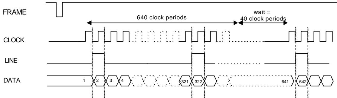
Frame signal is asserted low at the beginning of each frame.
