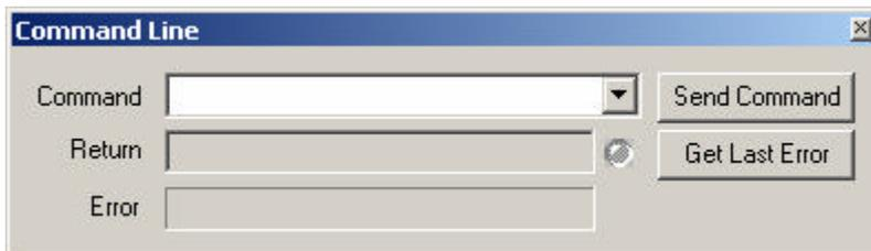
You must type the command : “DPI,” and push the button “Send Command”. In result, all BPR are deactivate in the current table of the camera. If this action have no error, the return from the camera is “DPI,1,”.
