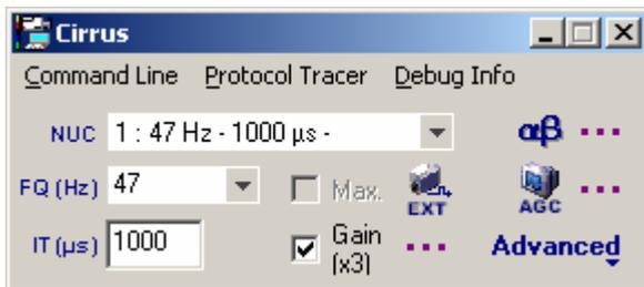
The “Command Line” menu will prompt the following window and allow you to send ASCII command line through an editor :
