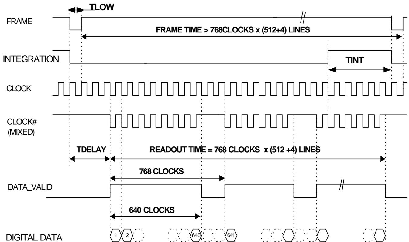
**TCLOCK** Digital pixel clock period 31.25ns Min to 50ns Max fréquency in 20MHz to 32MHz Max
