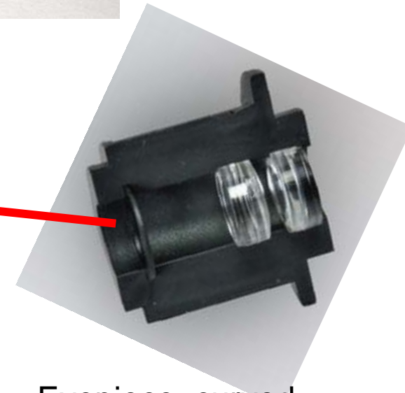
Eyepiece, curved sides face in, flat sides face out
