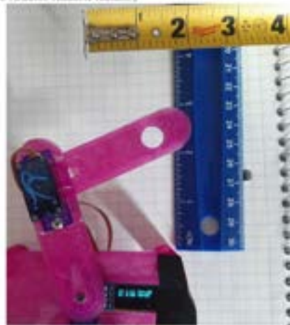
Figure 3: The robot in forward kinematics mode displaying the coordinates of the center of the hole after being commanded to move both joints to specific angles.
